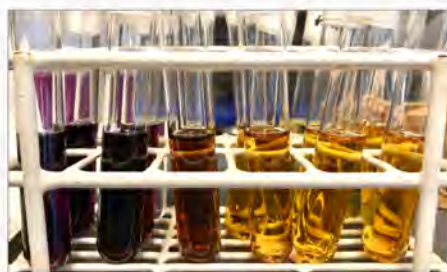
Figure 2: Test tubes for DPPH radical scavenging assay. From left to right: increasing concentrations of EEP, with constant concentration of DPPH. When the DPPH free radical is scavenged, or trapped, by a single electron donor, the solution turns yellow, losing its purple color. The more purple the solution, the less effective the antioxidant.
